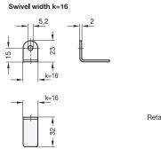
Clamp mounting GN 478 Retaining plate
